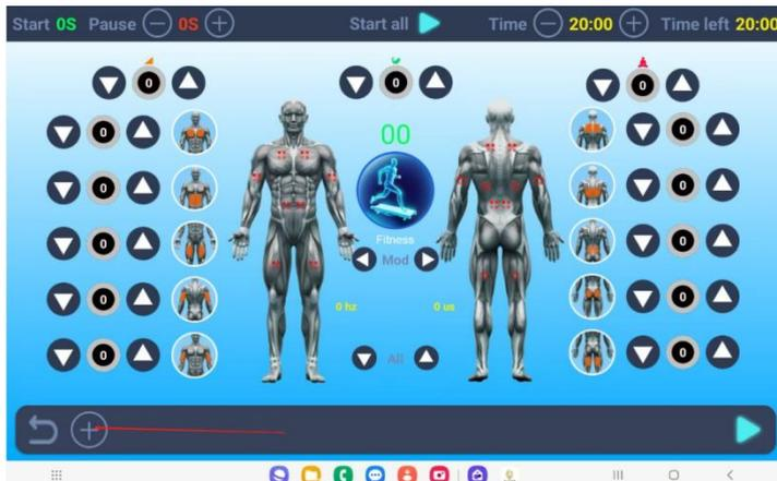
C. Select the energy box with the same number as your energy box, and click until you hear a beeping sound from the energy box and the light bar flashes. This means that pairing mode is activated.
